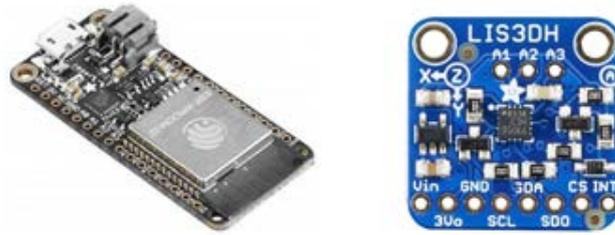
**Figure A.9 — SP32 board and Lis3DH on a breakout board**
